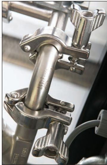
Triclamp fittings provide clean connections and complete modularity for easy servicing
